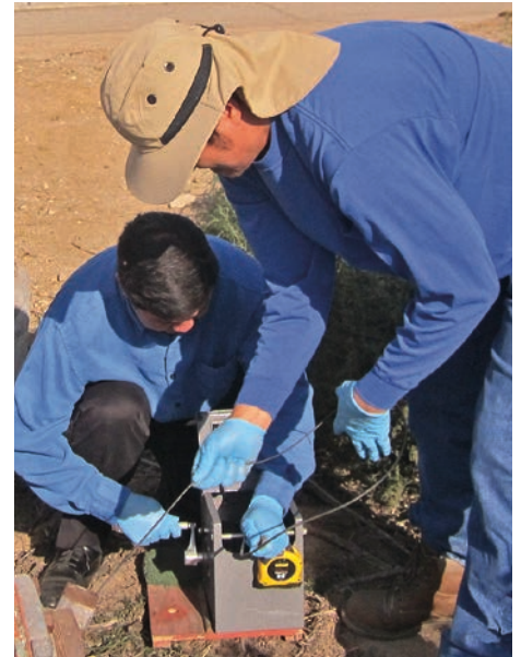
Watermaster staff performing groundwater level sampling.
